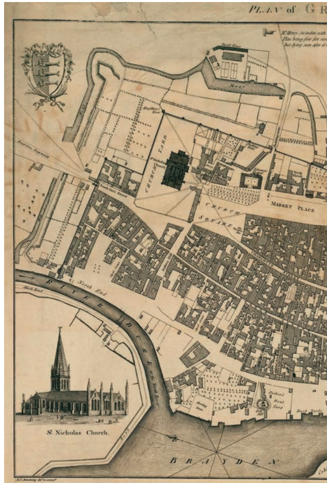
FIG. 904. DETAIL FROM MOSTYN JOHN ARMSTRONG, PLAN OF GREAT YARMOUTH, SURVEY'D BY THE LATE M r . HENRY SWINDEN , 1779. Scale, 1:2,376. Building shapes are mapped with considerable care in this example of eighteenth-century British town mapping by a local surveyor, the antiquary Swinden, who performed his survey as part of his research on the Roman town of Gariannum. The inscription states that this printed version is a reduction by Armstrong of Swinden's original manuscript plan of Gariannum, measuring two feet four inches by four feet nine inches (71 × 145 cm). Comparatively few towns were mapped in such detail. Size of the entire original: 54 × 73 cm; size of detail: ca. 38.5 × 26.0 cm. Image courtesy of the Museo Naval de Madrid (MN 138-28).
