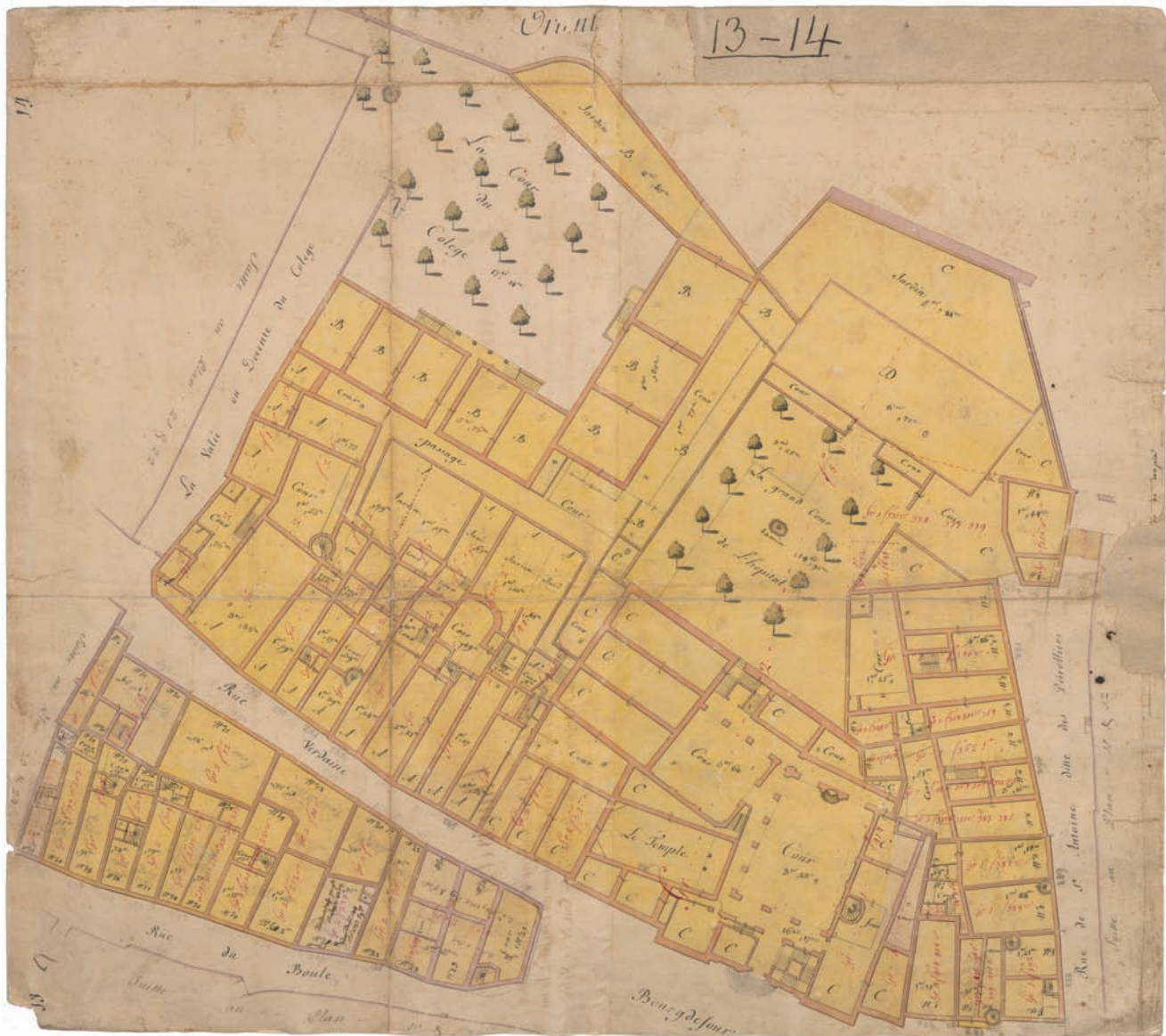
FIG. 934. "PLAN BILLON" OF GENEVA, 1726, SECTION 13–14. One of thirty-four manuscript sheets at a scale of 1:240 accompanied by a general plan at 1:800. These cadastral plans were commissioned by the government of the Republic of Geneva and surveyed by Jean-Michel Billon. Walls of structures
