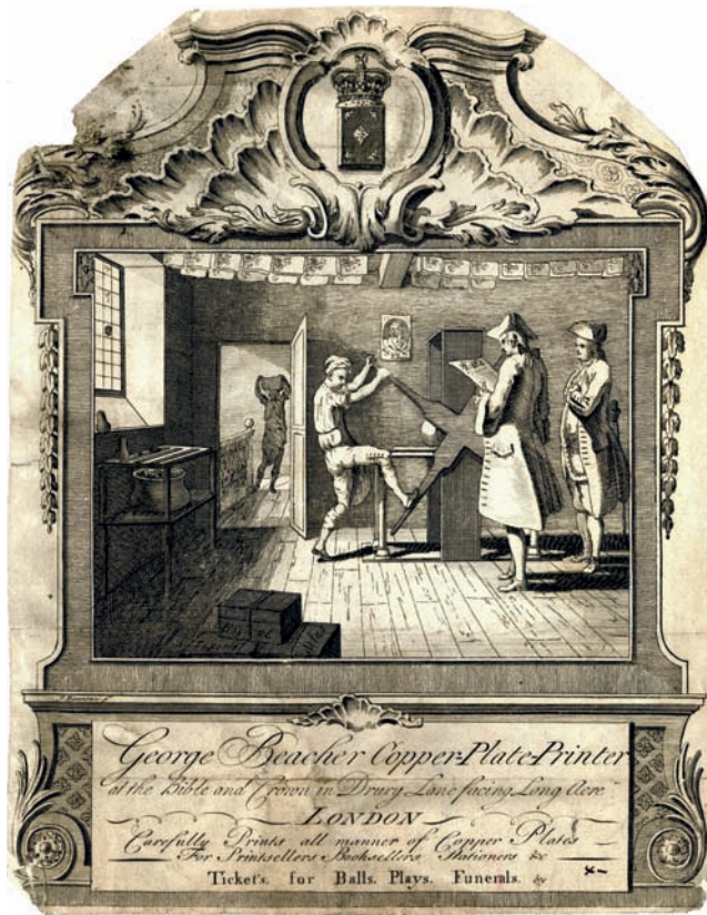
FIG. 722. TRADE CARD FOR GEORGE BEACHER, "COPPER-PLATE-PRINTER," 1740s. Engraved by Jacob Bonneau, the card shows Beacher's workshop with the roller press in action and prints hanging to dry above bales of different sizes of paper in the foreground; the inking table is to the left.
