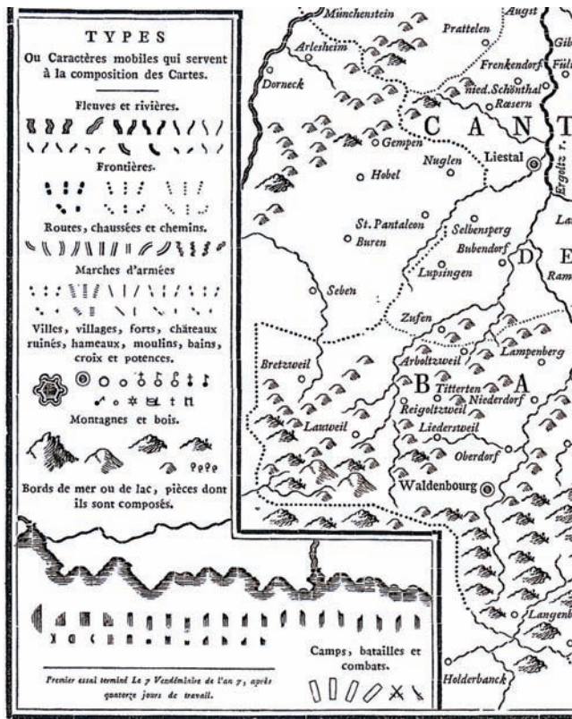
FIG. 727. DETAIL FROM THE CARTE TYPOMÉTRIQUE DU CANTON DE BASLE, 1798. The legend shows some of the different geographic fonts used to create the map. A further note on the map states that its first printing required fourteen days of work. Published by Wilhelm Haas, Son. Dedicated to one of the Cassinis, the map is dated using the French Revolutionary calendar: 7 Vendémiaire de l'an 7, i.e., 28 September 1798.
