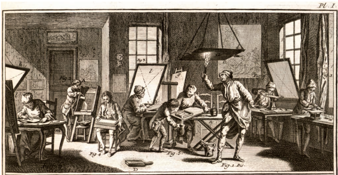
FIG. 718. ETCHING AND ENGRAVING IN A WORKSHOP. The following activities are labeled and described in the accompanying text: applying the ground with taffeta ball (fig. 1, far right); blacking the plate (fig. 1 bis); different techniques for applying acid to the plate or part of the plate (figs. 2, 4, 5); using the etching needle in copying the design, with diffused light from the chassis ( i ) (fig. 3); using the burin, with the cushion under the plate (fig. 6, lower left; label obscured by shadow); and hammering out mistakes (fig. 7, behind fig. 1). Detail from Denis Diderot and Jean Le Rond d'Alembert, eds.,
