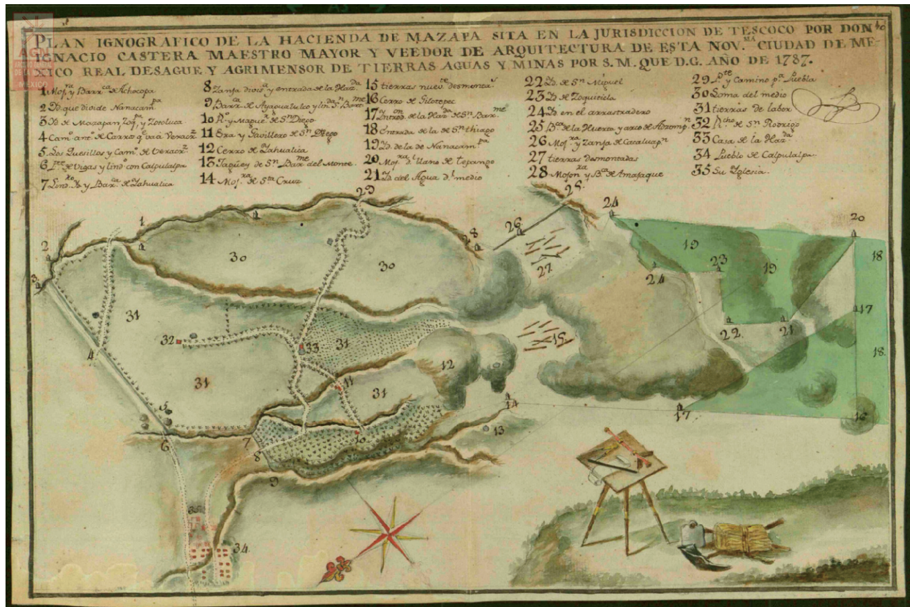
FIG. 47. IGNACIO CASTERA, "PLAN IGNOGRAFICO DE LA HACIENDA DE MAZAPA," 30 JANUARY 1787. This plan of a hacienda in Texcoco, near Mexico City, shows increased sophistication in mapping private property by emphasizing the accuracy of geometric calculations with the surveyor's table and tools laid out lower right.
