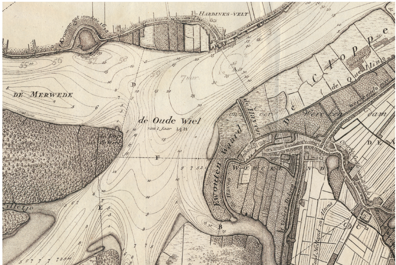
FIG. 33. DETAIL FROM NICOLAAS SAMUELSZ. CRUQUIUS, DE RIVIER DE MERWEDE, VAN (ONTRENT) DE STEENEN-HOEK (THE HAGUE, 1729–30). Copper engraving on two sheets; 1:10,000. Detail from sheet one showing the use of isobaths; these, and other data (see fig. 801) revealed that the Merwede had a very irregular depth and rate of flow, and that as much as two-thirds of the river's
