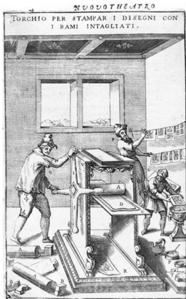
FIG. 22.9. INTAGLIO ROLLING PRESS. The rolling press relied on a different action than the letterpress screw press, providing intense pressure on plate and paper as they were passed through the rollers. Note the apprentice heating the copperplate before inking it.
